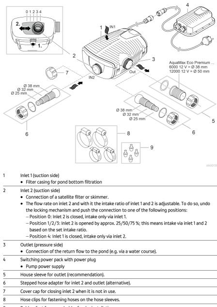
9 Rubber feet for pump holder for dry installation.
