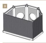
Important: Before moving on to step 13, ensure all the labels are removed from the panels, as you will be unable to remove them once the liner bag has been inserted.
